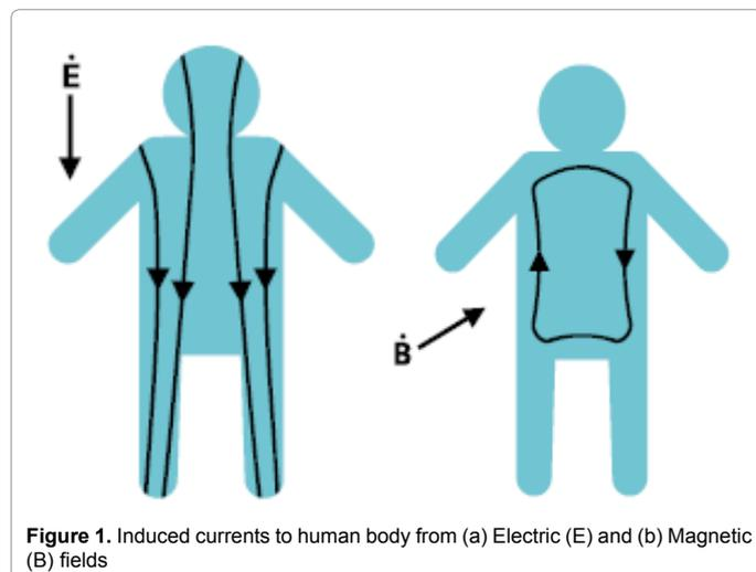
Figure 1. Induced currents to human body from (a) Electric (E) and (b) Magnetic (B) fields
