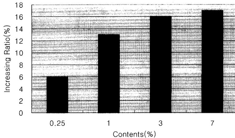
**Figure 3.** The increasing ratio of radiation energy ( $W/m^2$ ) of the O/W emulsion containing the tourmaline powder. The y-axis is the increasing ratio (percentile) and the x-axis is the contents of the tourmaline powder.
