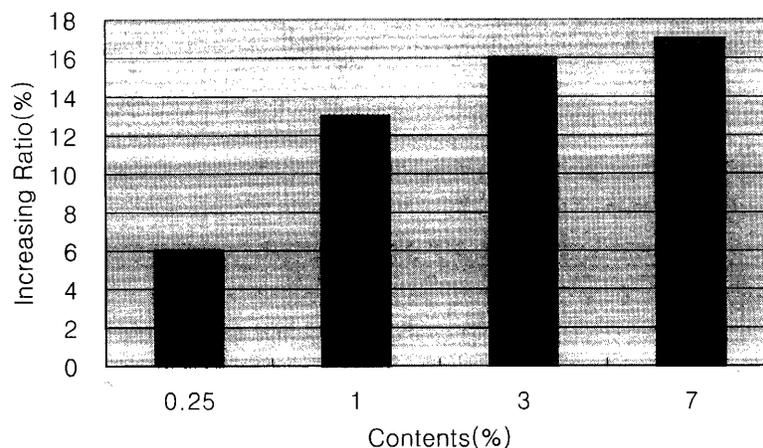
**Figure 4.** The increasing ratio of radiation energy ( $W/m^2$ ) of the O/W emulsion containing the jade (nephrite) powder. The y-axis is the increasing ratio (percentile) and the x-axis is the contents of the jade (nephrite) powder.
